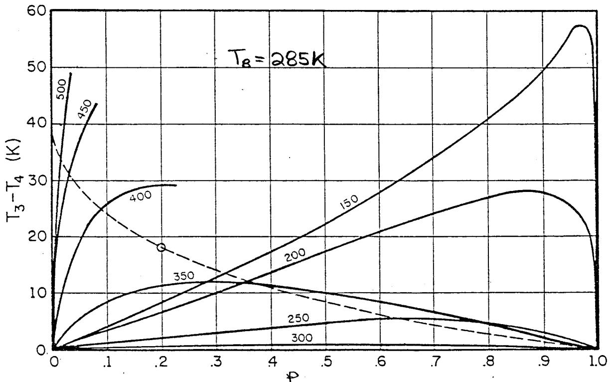
4.  $T_3 - T_4$  vs.  $p$  for increasing values of  $T_t$ , for  $T_b = 285$  K. Curves terminate where either sensor would saturate. The dashed line shows the range of values permissible when  $T_3 = 325$  (but is only applicable for values of  $T_t$  which are greater than  $T_b$ ).
