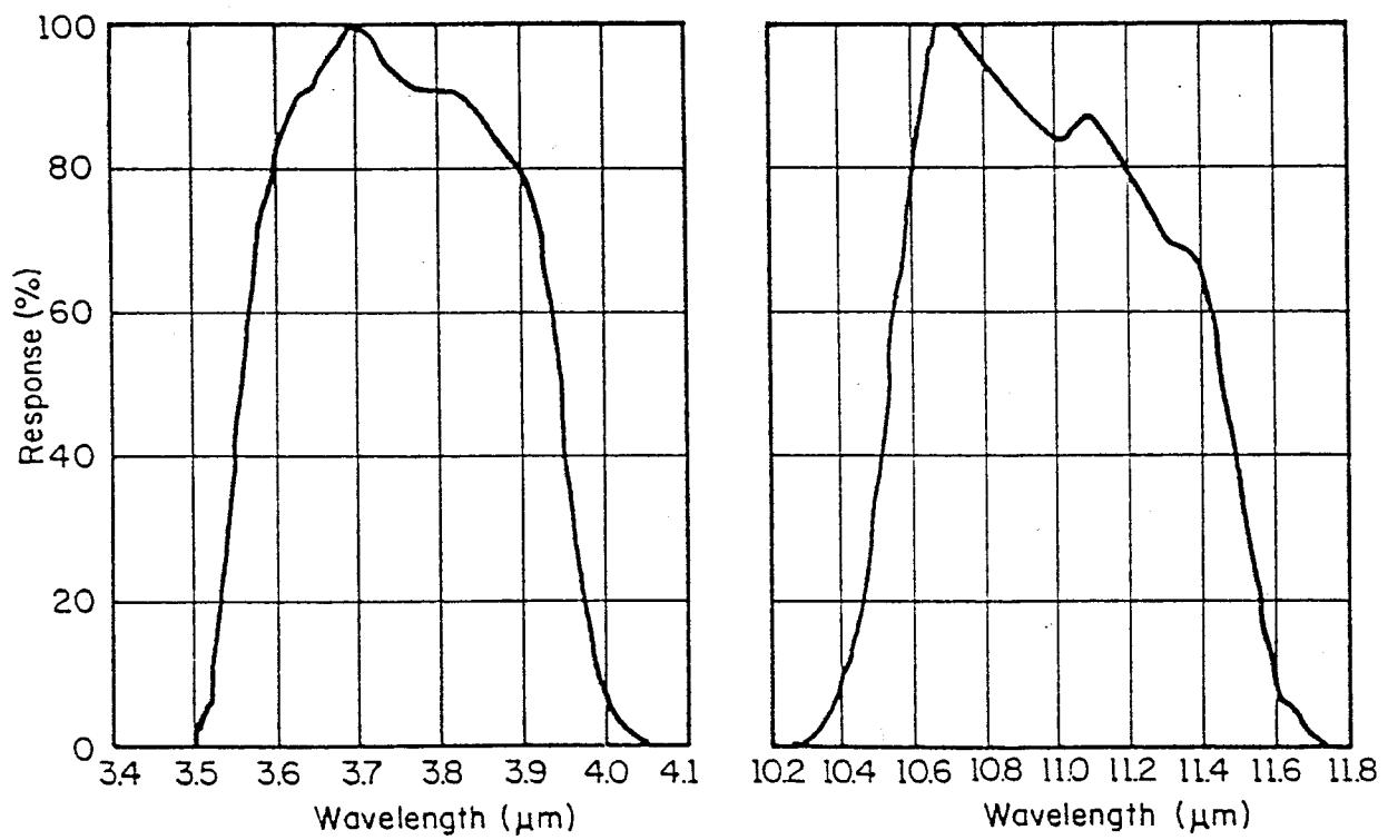
1. Relative spectral response functions (per cent) for channels 3 (left) and 4 (right) of the NOAA-6 satellite (from Kidwell, 1979).
