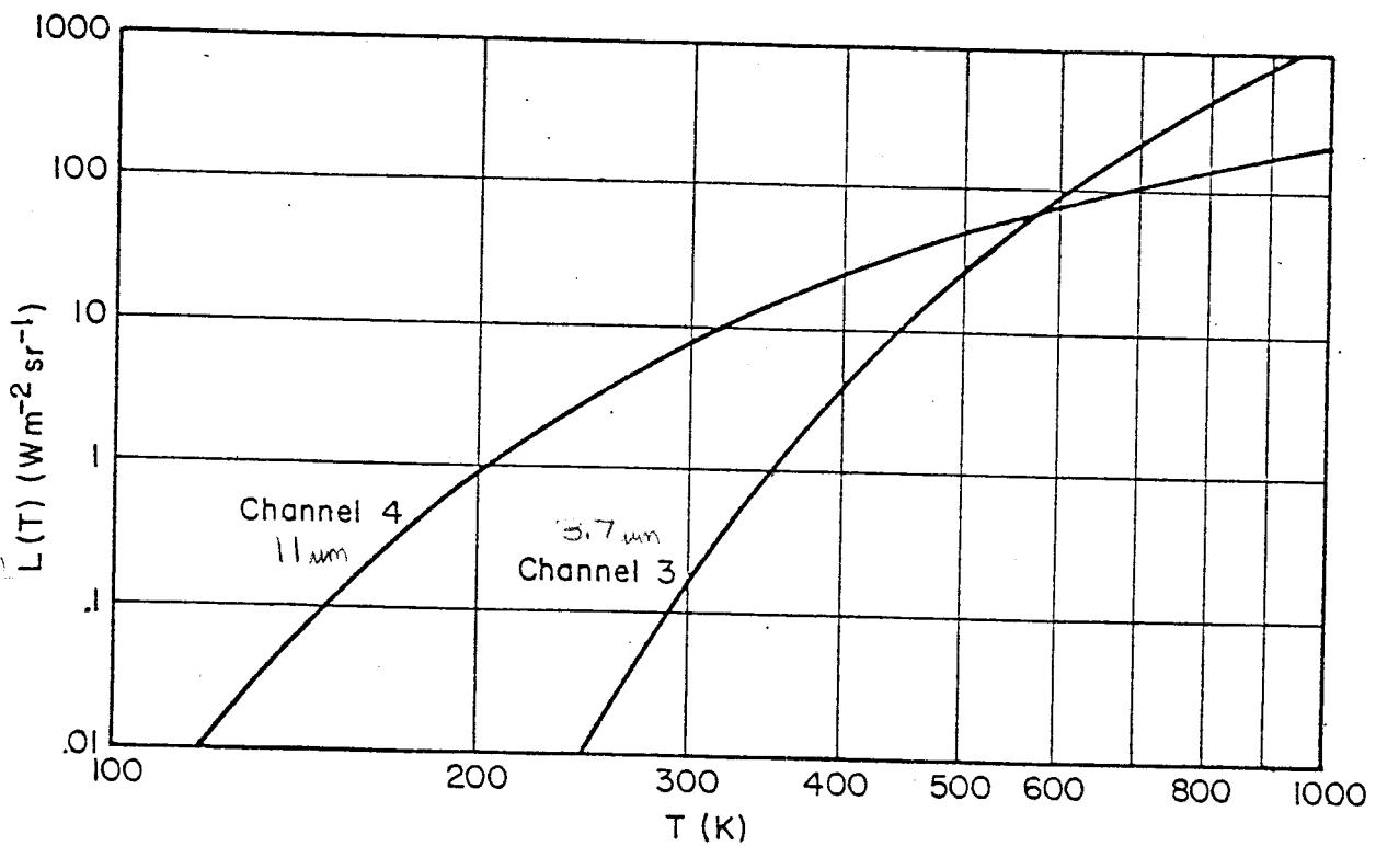
2. NOAA-6 radiances for channels 3 and 4 vs. temperature, as calculated by eq. (1) with the spectral response functions in figure 1.
