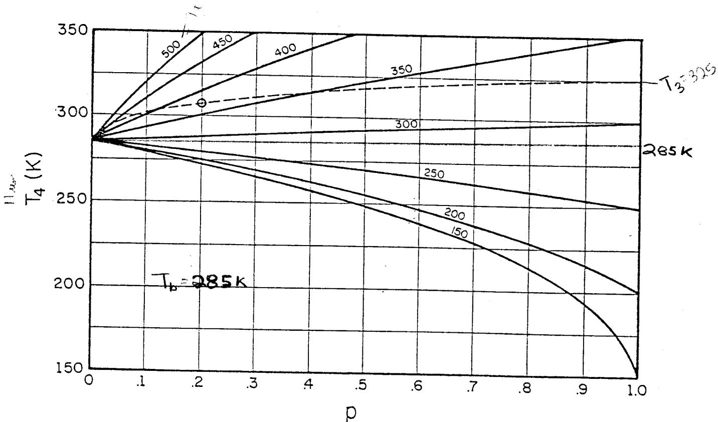
3.  $T_3$  (top) and  $T_4$  (bottom) vs.  $p$  for increasing values of  $T_1$ , for  $T_b = 285$  K. The dashed line in the lower graph shows the range of values permissible when  $T_3 = 325$ .
