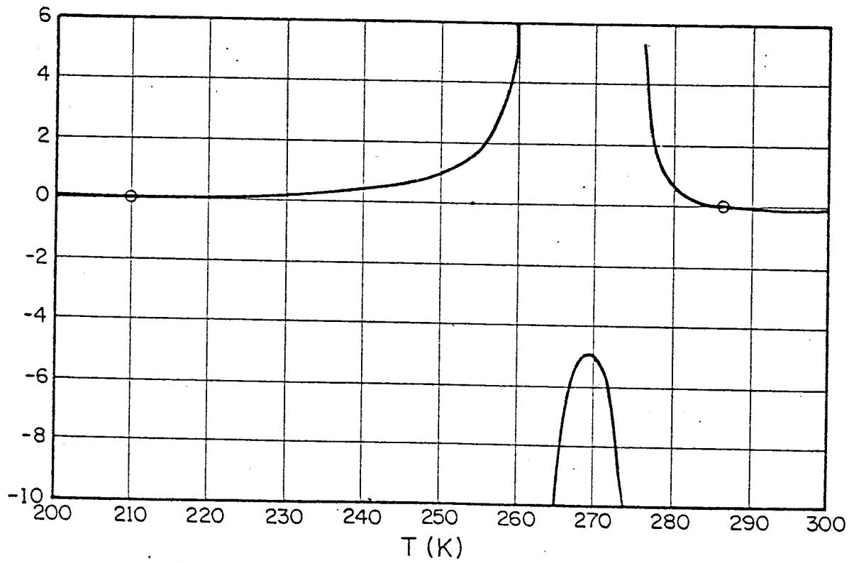
5. Graph of eq. (8) for  $T_3^{(1)} = 261.4$ ,  $T_3^{(2)} = 274.6$ ,  $T_4^{(1)} = 241.5$ , and  $T_4^{(2)} = 262.9$ . The solutions are  $T_b = 210$  and  $T_i = 285$ .
