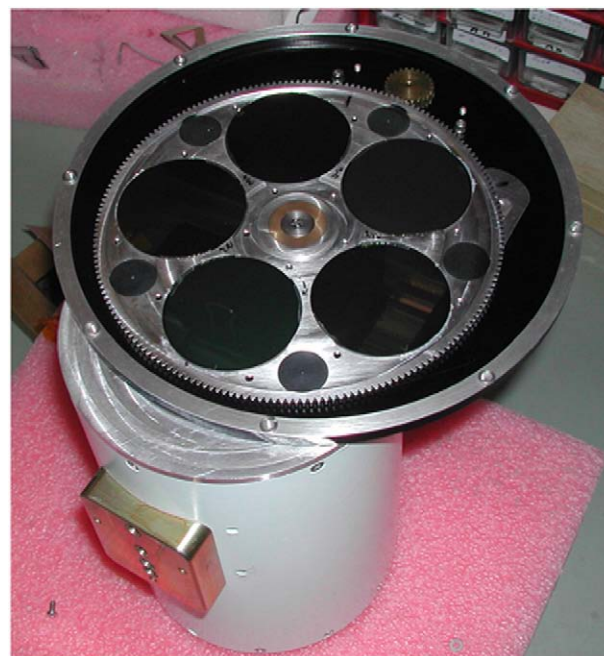
Fig. 1. Cyclops filter wheel and interference filters. The current arrangement has 5 filters with central wavelengths at 7.34, 8.55, 10, 11, 12 \mu\text{m} . For operations from the ground, the 7.34 \mu\text{m} filter was replaced with a broadband filter covering 7\text{--}14 \mu\text{m} .
