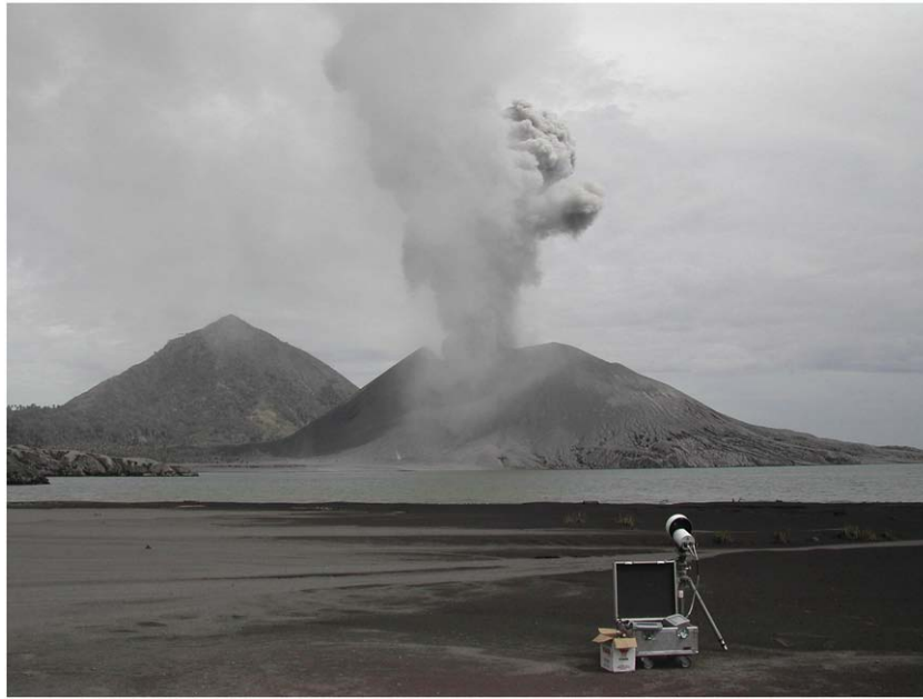
Fig. 15. Photograph of Cyclops at Rababa “hot springs” during a measurement sequence and nearly continuous ash eruption activity.
