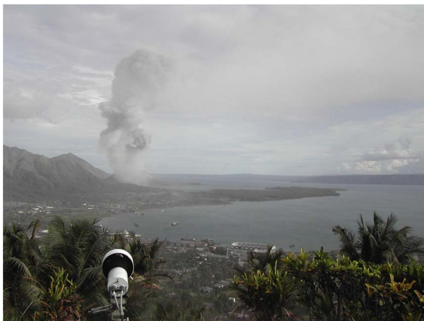
Fig. 13. Photograph of the Cyclops camera viewing an eruption column from Tavurvur, Rabaul, New Britain. The camera is approximately 7 km from the erupting volcano.
